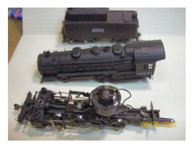
A flash-why not convert it to DCC? With the multimeter and the test power, I discovered the electrical layout. The manufacturer's specs said it was rated for 12VDC at 0.4A maximum. There would be room in the firebox for a z-scale DCC decoder.
