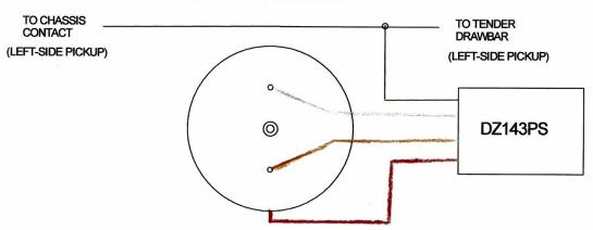
LEFT-SIDE WIRES REMOVED FROM MOTOR CONTACT AND CONNECTED TO DZ143PS BLACK WIRE. MOTOR SHELL DISCONNECTED FROM MOTOR CONTACT AND CONNECTED TO DZ143PS RED WIRE. DZ143PS ORANGE WIRE CONNECTED TO RIGHT-SIDE MOTOR CONTACT. DZ143PS GRAY WIRE CONNECTED TO LEFT-SIDE MOTOR CONTACT.
